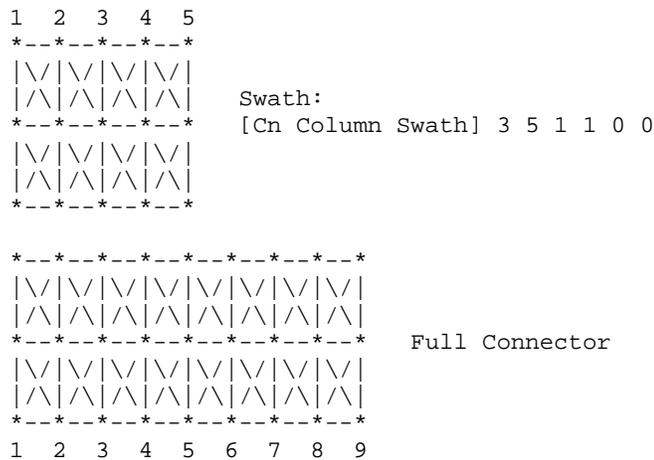
The matrix data for swath columns 1 and 2 (including forward references) copied into the new full connector matrix.
