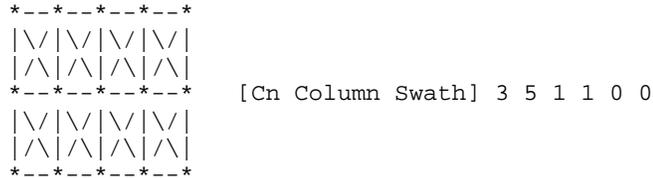
Notice that columns 2, 3, and 4 have the maximum amount of coupling from each side. In this case the edge effect columns 1 and 5 do not have coupling from both sides.
