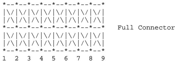
The Swath above is centered about column 4. The paths of interest including those of columns 3 and 5 are also described by swath matrix data that has coupling from both sides. However, because of edge effects, columns 2 and 6 are less accurately approximated.
