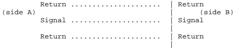
The return path must include all pins that are power or ground. In a loop inductance matrix, the diagonal terms represent the loop inductance of a specific pin with return currents assumed returned through all pins defined to be power or ground.
