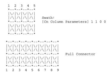
Starting at the center of the swath, the coupling pattern of just the center column (column 3 in this example) is copied for the connector matrix. In this case, the coupling pattern extends forward to the next column. The pattern is copied by mapping the swath pin numbers into the connector pin numbers and copying the center column forward referenced data. In this example, the operation starts at the full connector column 3 and ends upon completion at the full connector column 7.
