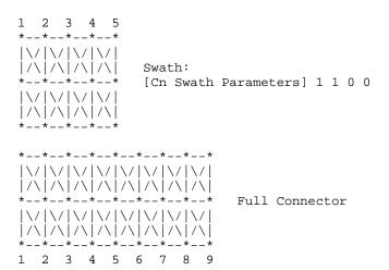
The Swath above is centered about column 4. The paths of interest including those of columns 3 and 5 are also described by swath matrix data that has coupling from both sides. However, because of edge effects, columns 2 and 6 are less accurately approximated.
