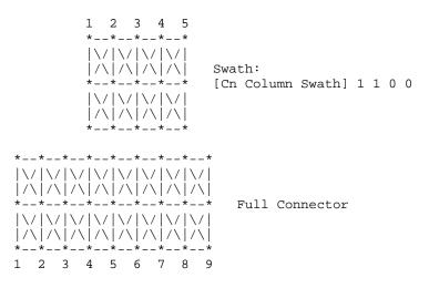
The final step is similar to Step (a), but concluded using the right side of the swath. When the swath is positioned against the right edge as shown, then the coupling patterns for the swath columns are duplicated for the final columns of the full sized connector. So the patterns of swath columns 4 and then 5 are duplicated for the full sized connector columns 8 and 9.
