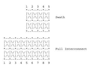
The final step is similar to Step (a), but concluded using the right side of the swath. When the swath is positioned against the right edge as shown, then the coupling patterns for the swath columns are duplicated for the final columns of the full sized interconnect. So the patterns of swath columns 4 and then 5 are duplicated for the full sized interconnect columns 8 and 9.
