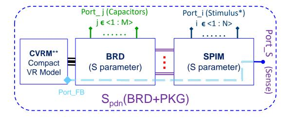
\*The impedance, measured at the Port\_FB differential pair, is equivalent to that observed at the observing port (Port\_S), which is usually located somewhere in package.
