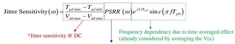
Frequency dependency due to PSRR (Power Supply Rejection Ratio)
