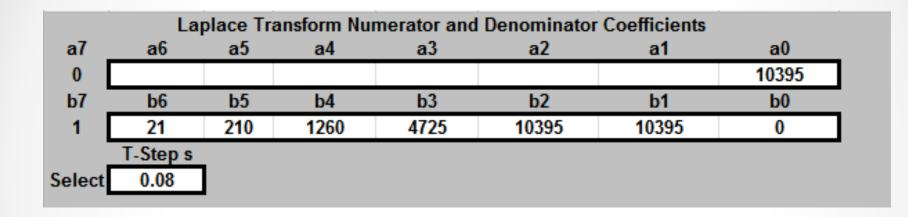
**Convert all-pass to low-pass filter by zeroing out numerator coefficients (click/back-space or enter 0) for real-time modification**
