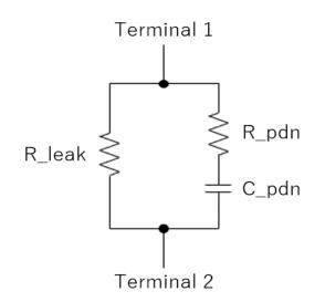
PDN networks are simply described, and connect between signal names or bus labels (terminals) described as PDN Domains
