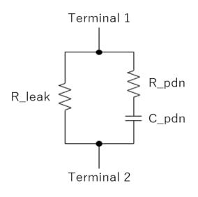
PDN networks are simply described, and connect between signal names or bus labels (terminals) described as PDN Domains
