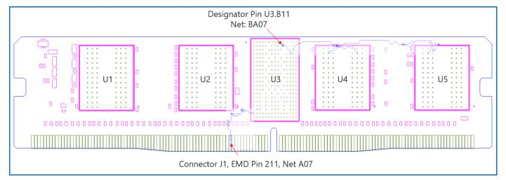
Four devices here are instances of a single IBIS component
