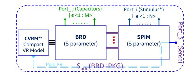
\*The impedance, measured at the Port\_FB differential pair, is equivalent to that observed at the observing port (Port\_S), which is usually located somewhere in package.
