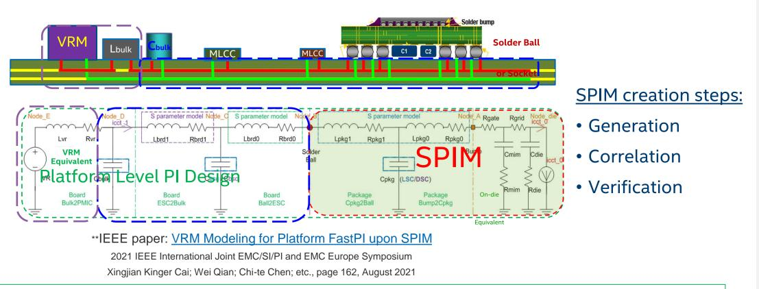
• **SPIM:** Standardized PI Model, for each power rail in a SoC/PKG, or a module.
