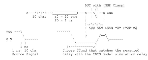
Example of TTgnd Extraction Setup
