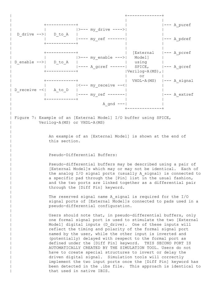
The D\_to\_A adapters used for SPICE, Verilog-A(MS) or VHDL-A(MS) files can be set up to control ports on pseudo-differential buffers. If SPICE, Verilog-A(MS) or VHDL-A(MS) is used as an external language, the [Diff Pin] vdiff subparameter overrides the contents of vlow and vhigh under A to D.
