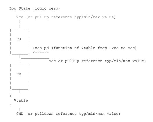
The effective current table for the Isso\_pu current is extracted by the following process. The buffer is set to "logic one". A Vtable voltage source is inserted between the [Pullup Reference] node and the buffer as shown below. This Vtable voltage is swept form -Vcc (typical) to +Vcc (typical) and is relative to the [Pullup Reference] typ/min/max values for the corresponding columns. The output is connected to the Vcc (typical) value as shown below.
