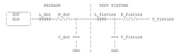
NOTE: The use of L\_dut, R\_dut, and C\_dut is strongly discouraged in developing waveform data from simulation models. Some simulators may ignore these parameters because they may introduce numerical time constant artifacts.
