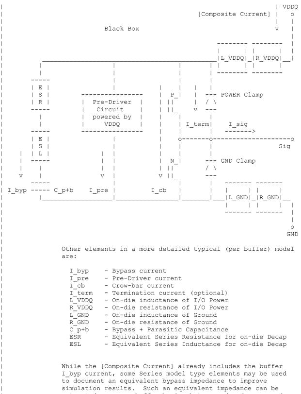
[Rc Series] and [R Series] under a separate [Model]. These elements are connected using the [Series Pin Mapping] keyword. Paths between several voltage rails can be modeled in this manner. The [Pin Mapping] keyword documents what buffers share common and often isolated power rails.
