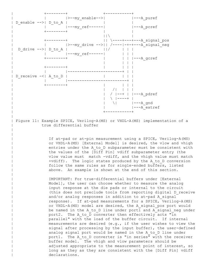
Note that the thresholds refer to the state of the non-inverting signal, using the inverting signal as a reference. Therefore, the output signal is considered high when, for example, the non-inverting input is +200 mV above the inverting input. Similarly, the output signal is considered low when the same non-inverting input is -200 mV "above" the inverting input.
