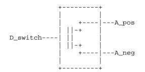
Figure 3: Port names for series switch
