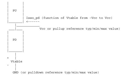
The effective current table for the Isso\_pu current is extracted by the following process. The buffer is set to "logic one". A Vtable voltage source is inserted between the [Pullup Reference] node and the buffer as shown below. This Vtable voltage is swept form -Vcc (typical) to +Vcc (typical) and is relative to the [Pullup Reference] typ/min/max values for the corresponding columns. The output is connected to the Vcc (typical) value as shown below.
