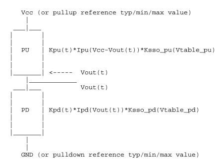
The Vtable\_pd and Vtable\_pu values may change at each time step. The Ksso\_pd(Vtable\_pd) and Ksso\_pu(Vtable\_pu) values are derived from the dynamic reference voltage variation and [ISSO PD] and [ISSO PU] table entries according to the formulas below: Ksso\_pd(Vtable\_pd) = Isso\_pd(Vtable\_pd)/Isso\_pd(0)
