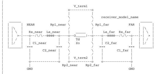
If the Td subparameter is present, then the Zo subparameter must also be present. If the Td subparameter is not present, then the simulator must remove the transmission line from the network and short the two nodes to which it was connected.
