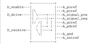
Figure 10: Port names for true differential I/O buffer
