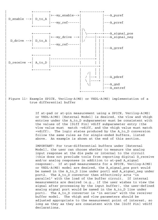
Note that the thresholds refer to the state of the non-inverting signal, using the inverting signal as a reference. Therefore, the output signal is considered high when, for example, the non-inverting input is +200 mV above the inverting input. Similarly, the output signal is considered low when the same non-inverting input is -200 mV "above" the inverting input.
