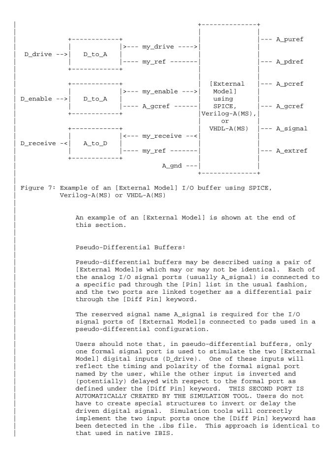
The D\_to\_A adapters used for SPICE, Verilog-A(MS) or VHDL-A(MS) files can be set up to control ports on pseudo-differential buffers. If SPICE, Verilog-A(MS) or VHDL-A(MS) is used as an external language, the [Diff Pin] vdiff subparameter overrides the contents of vlow and vhigh under A\_to\_D.
