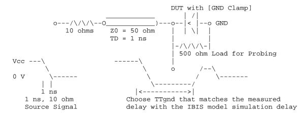
Example of TTgnd Extraction Setup
