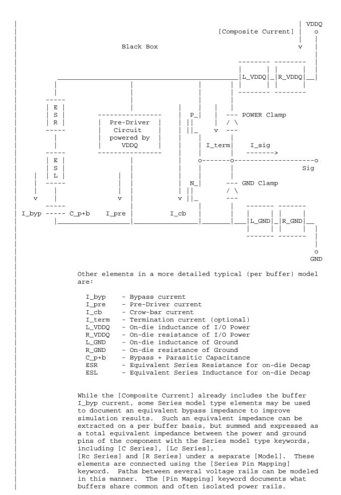
The C\_p+b value might include the detailed distribution of C\_comp when C\_comp\* is attached to several rails. If the C\_comp value and the C\_p+b value are about the same magnitude, the [C Series] value should be adjusted to avoid double counting.
