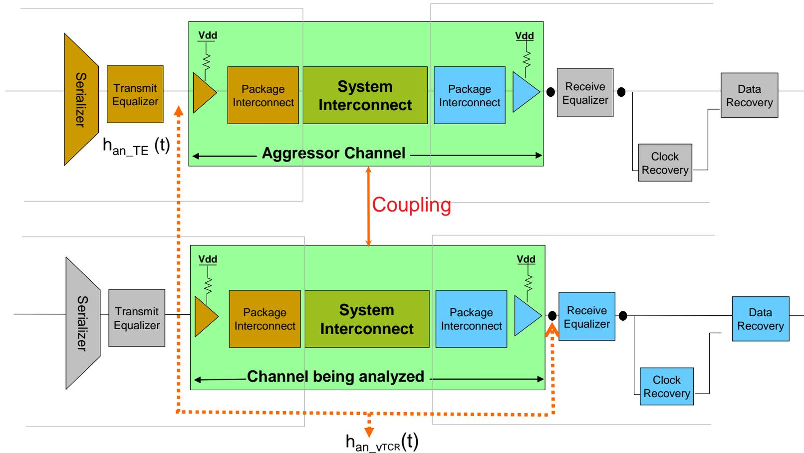
$h_{an\_TE}(t)$  = Impulse Response of Aggressor's TX Equalization
