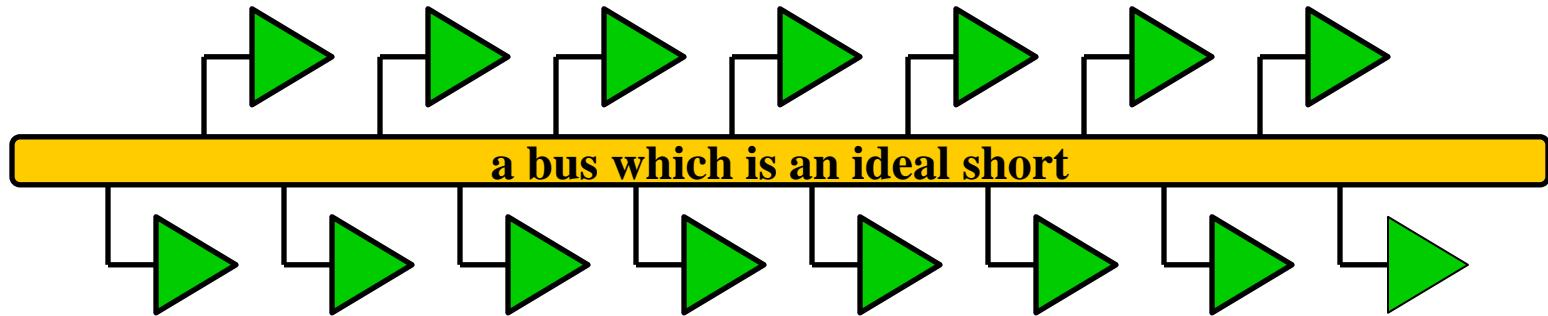
If the “bus” is an ideal short, each receiver sees exactly the same signal, i.e. the bus is just a node
