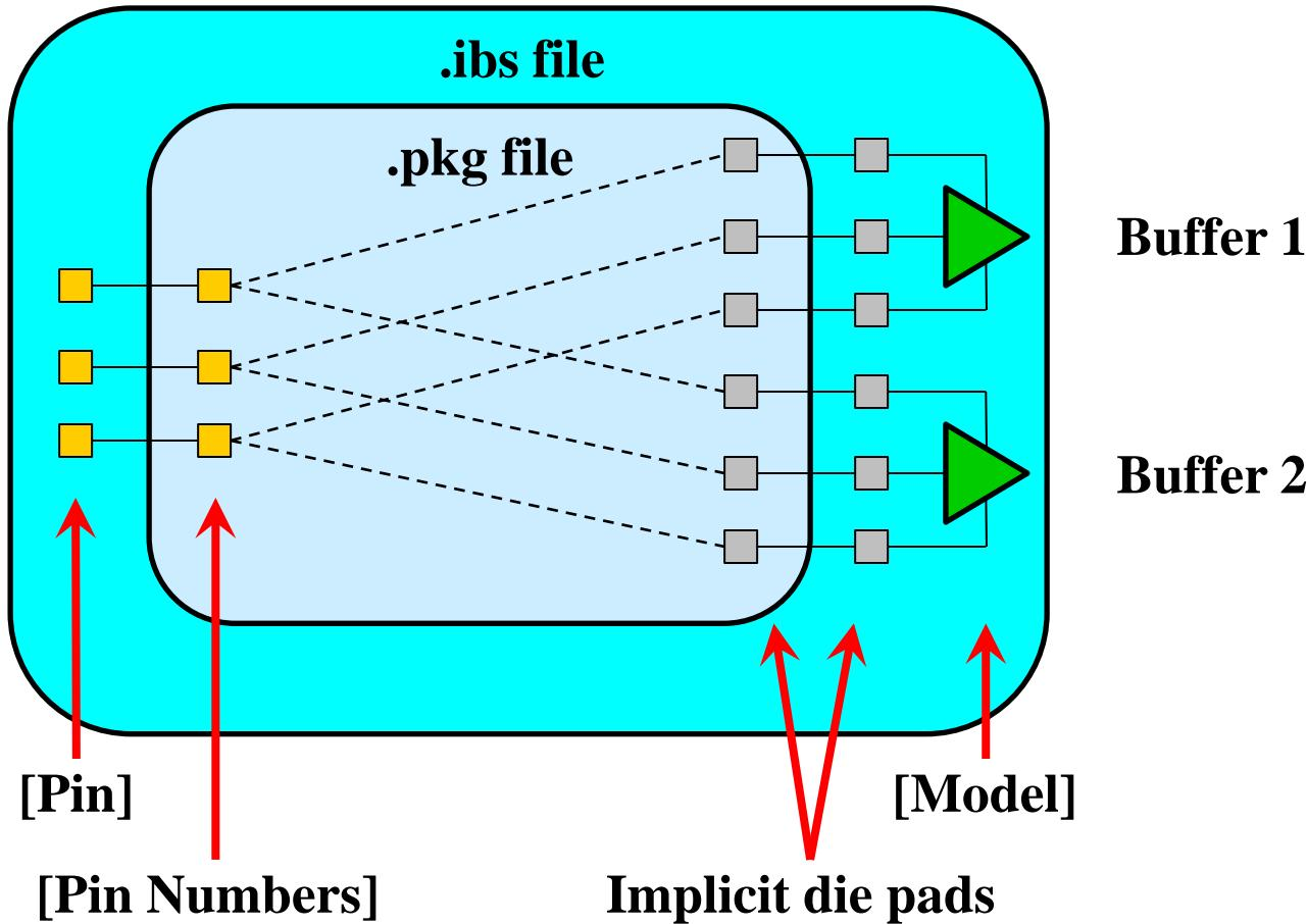
Buffers are “instantiated” by the 3<sup>rd</sup> column of the [Pin] keyword.
