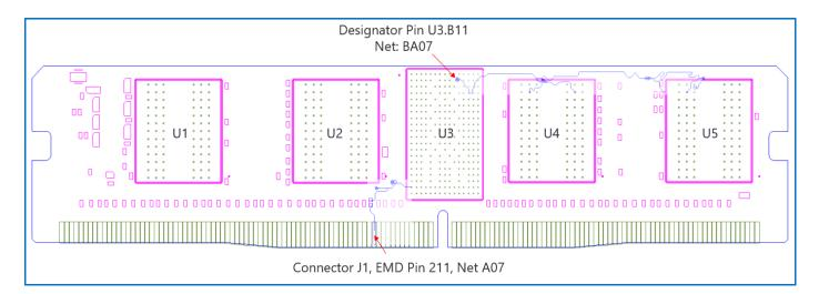
Four devices here are instances of a single IBIS component
