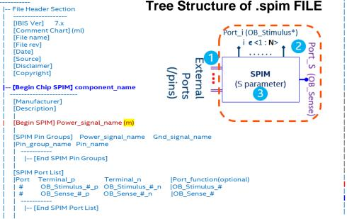
[SPIM Touchstone File Name] \_\_\_\_\_ [SPIM Stimulus] OB Stimulus Weighting ------- [End SPIM Stimulus] [SPIM Target] [SPIM Observation Port] Frequency Z(typ) Z(min) Z(max) \_\_\_\_\_ |-- [End SPIM Target] [SPIM Rnetwork File Name] \_\_\_\_\_ [SPIM Current] ll(name) l(type) l(min) l(max) \_\_\_\_\_ |-- [End SPIM Current] [Voltage List] V(name) V(typ) V(min) V(max) |-- [End Voltage List] [End SPIM] Power\_singal\_name [End Chip SPIM] component name [End]
