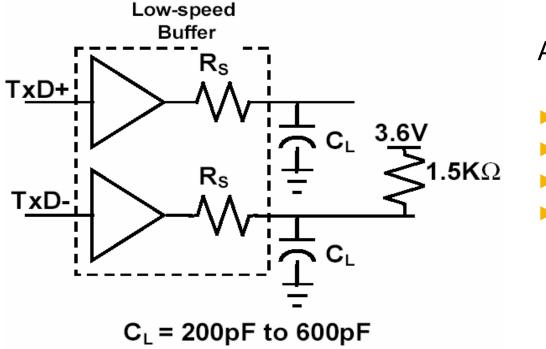
AC Test Load Conditions.
