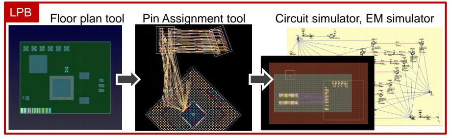
LPB has module's physical shape data and layout data. die outline, PKG outline, die pad shape, PKG ball shape, etc. P/G plane shape, transmission line shape, layer stackup, etc. And, these modules are linked to IBIS models or other models. LPB makes it easy to proceed design phase.
