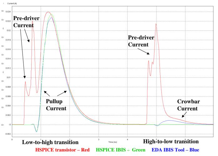
The total VDDQ current for the transistor-level model is significantly different from its pullup component. There is a large amount of pre-driver current due to crowbar effects and gate capacitance charging.
