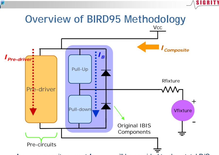
A new composite current I<sub>Composite</sub> will be provided to show total P/G currents, based on transistor simulation, for better P/G noise simulation
