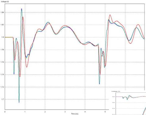
SSO waveforms with realistic PDS, 10 pF driver load, PWL I(t) in parallel with the IBIS device
