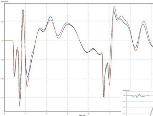
The IBIS simulations now show excellent correlation with the SPICE results over the full simulation. With the addition of the RC circuit, the oscillations occur at the proper frequencies and the SSO magnitude is correct.
