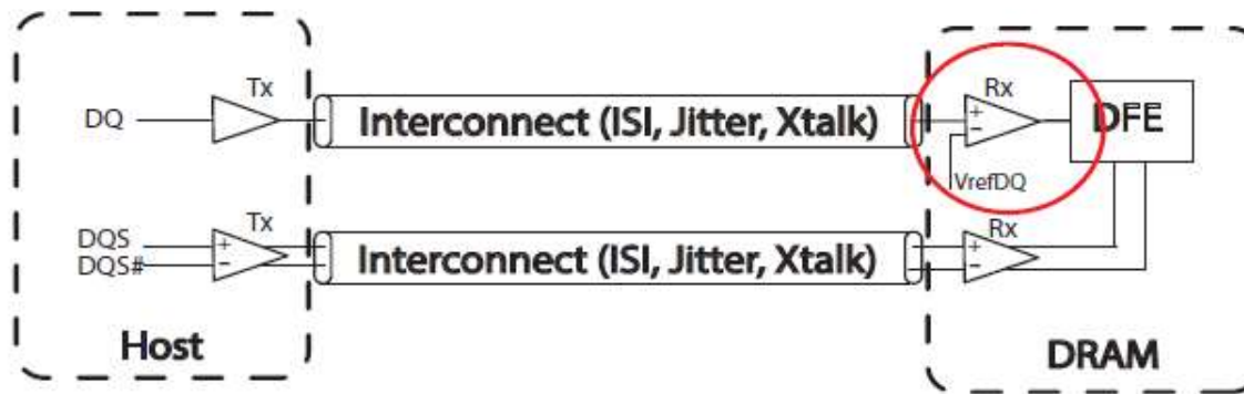
Figure 154 — Example of Rx Stressed Test Setup in the Presence of ISI, Jitter and Crosstalk
