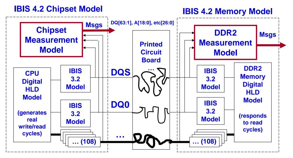
\* Note: This model is not in strictly IBIS 4.2 compliant because it uses an external circuit that references an IBIS 3.1 model
