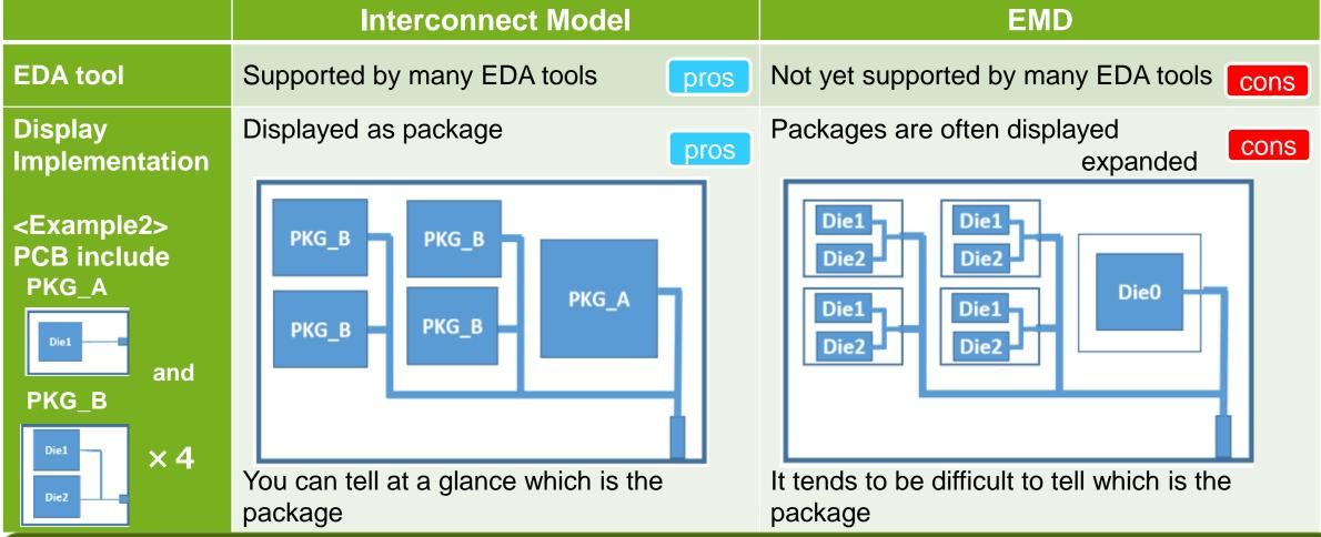
Many EDA tools does not support the EMD model at this time In EMD (similar to EBD) is difficult to distinguish between the package and the PCB
